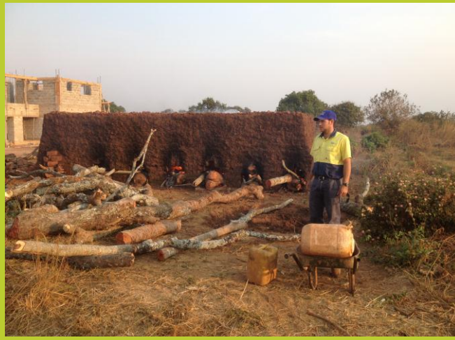
A local kiln is used to bake the bricks. Women used their hands to dig out gravel, taking 4 hours to gather a trailer load. TTN team members and community members dug trenches to begin foundations for the new clinic and school buildings.
